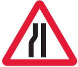
**Road narrows ahead** – sign warns the driver which side of the carriageway is obstructed. Place it between the ‘Road works ahead’ sign and the beginning of the lead-in taper. Make sure that the correct sign (i.e. narrows on left or right) is used.
