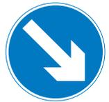
**Directional arrow** – place ‘Keep right’ or ‘Keep left’ signs as appropriate at the beginning and end of the lead-in taper of cones. These signs must be the same size as the ‘Road works ahead’ sign. Make sure that the signs point in the correct direction.
