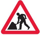
**Road works ahead** – the first sign to be seen by approaching traffic. Its size, the minimum distance from the start of the lead-in taper, and clear visibility distance will vary according to the type of road and its speed limit – see table inside the back cover. The range of distances is given to allow the sign to be placed in the most convenient position, bearing in mind the available space and visibility for drivers. Do not simply choose the minimum distance – assess each site carefully.
